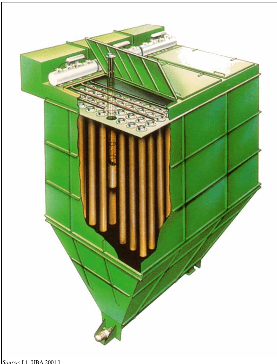
Figure 2.35: An example of a bag filter
